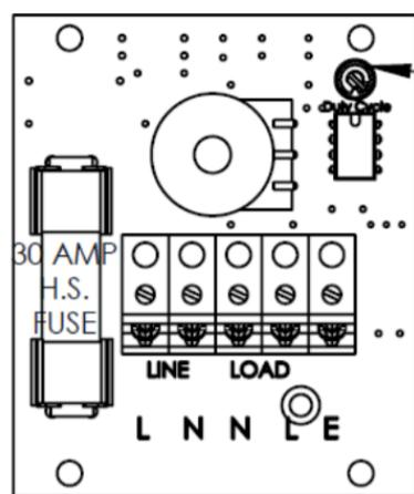
CAUTION: Use insulated trimmer to adjust cermet for required duty cycle.
